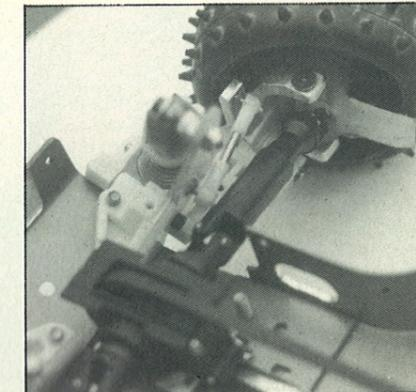
Above: RC10 wishbones and dampers have been retained and mated to Schumacher's excellent drive shafts, new hub carriers had to be machined using nylon 66.
