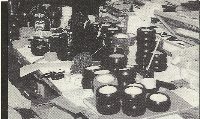
Masami Hirosaka had a production line set up for the tyres, he was using of split compounds glued together.
