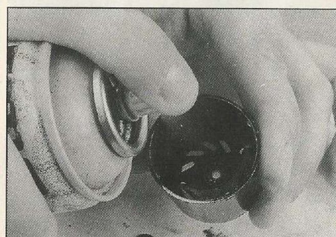
The can will also have collected a lot of dirt remove this first by brushing and then by spraying motor cleaner.
