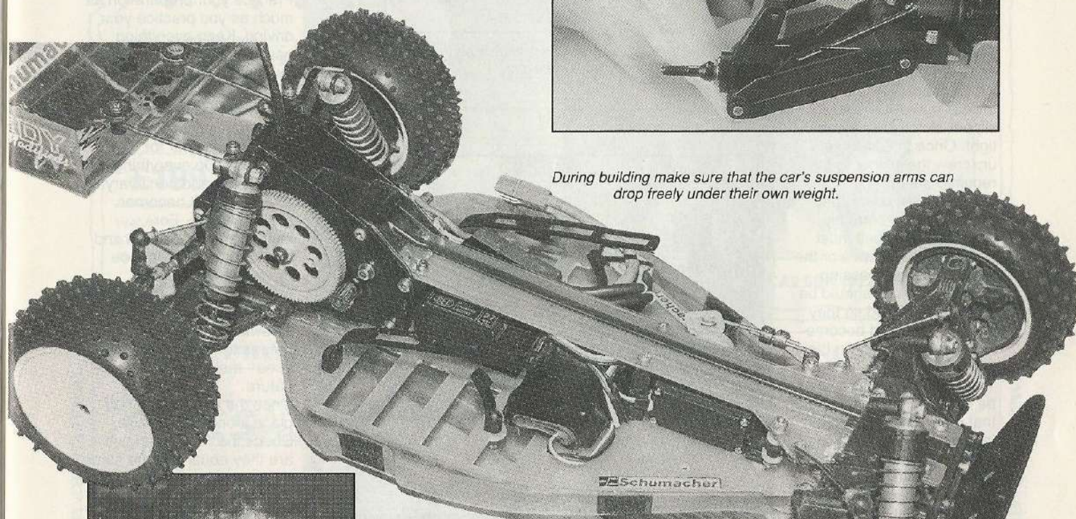
Left; Working on the car between heats is part of R/C car racing. Right; Make sure shock absorber springs are well seated.
