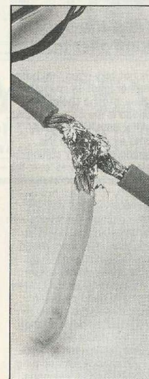
Left; Wiring like this causes shorts and therefore blow ups. Below; Holy crispy circuit boards Batman! a speedo well beyond repair.
