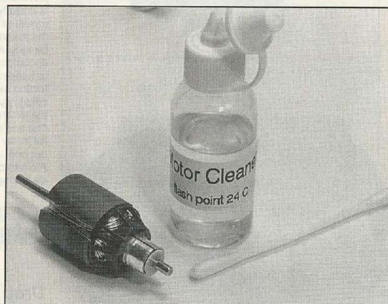
Some manufacturers offer a specialised motor cleaning fluid that will remove dirt without damaging the armature.
