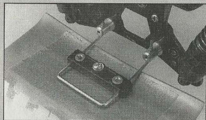
Tamiya's plastic wing mount is ideal, keeping the wing level and firmly in place.
