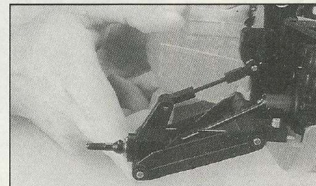
During building make sure that the car's suspension arms can drop freely under their own weight.
