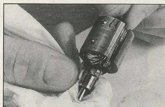
Clean the copper of the armature with a clean tissue and a spray of motor cleaner. Be careful and treat the armature gently as it is made from relatively soft material.
