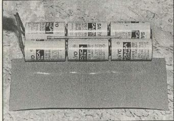
A piece of heat shrink cut to the correct size.
