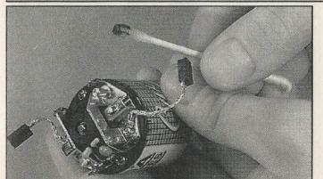
Ughh!!... the black dirt removed! Repeat this process until the copper colour of the armature shows through.
