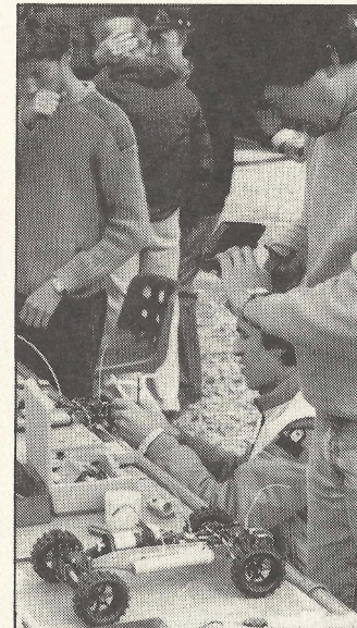
The SG/TAG 'Coyote' employs shaft drive between front and rear from an in-line motor. Ni-Cads are carried in two, three cell, sticks mounted either side of the chassis. Limited slip differentials feature front and rear.
