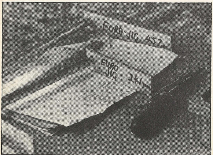
Below: measuring jigs to check dimensions of all competitors' cars against the EFRA construction rules.
