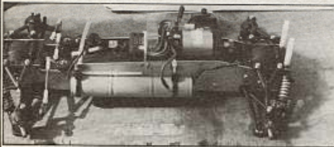
The SG/TAG 'Coyote' employs shaft drive between front and rear from an in-line motor. Ni-Cads are carried in two, three cell, sticks mounted either side of the chassis. Limited-slip differentials feature front and rear.
