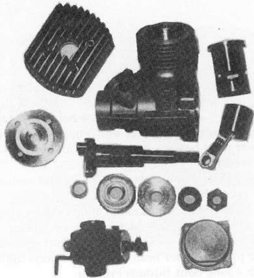
Stripped OPS Motor Showing Std Small Bore Carb & Heat Sink Head.
