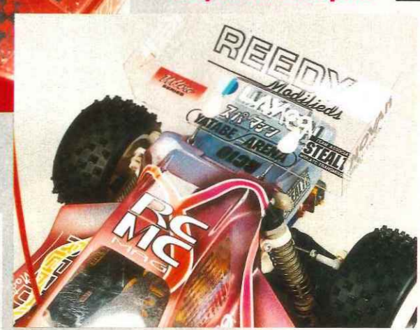
Craig uses the RCPS Turbo Mirage body on his RC10 - the body is very popular in the US. Note clover body post mounted through the body on the servo post.
