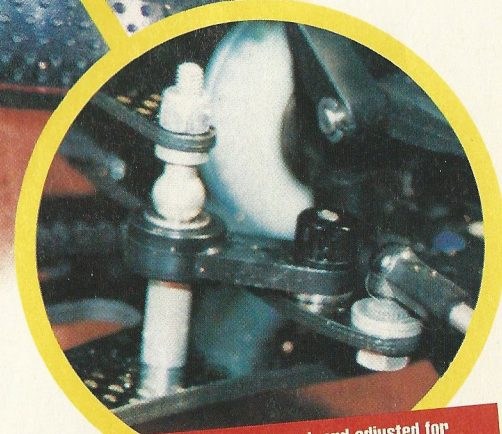
The steering is fully ballraced, and adjusted for "bump steer".
