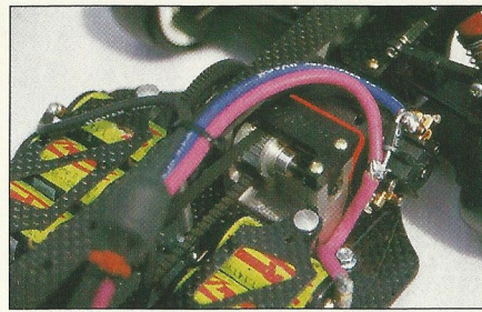
Duel drive is now available with the new layshaft, slide the collet to the right, either add or remove the drive pin.
