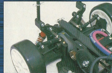
The M2 now has the YZ10 diffs, for a much higher drive ratio, more top speed. With the new "quick release" rear brace the car is much simpler to work on.
