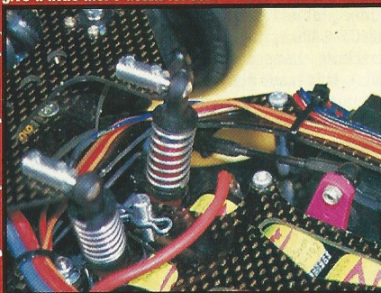
Try and keep the wiring neat as it has to cross over the main chassis plate.
