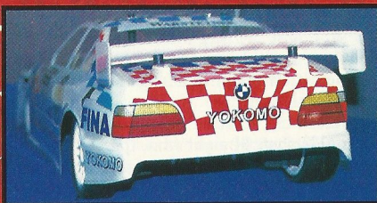
Note the spacers included under the rear wing, these give a little more down force.
