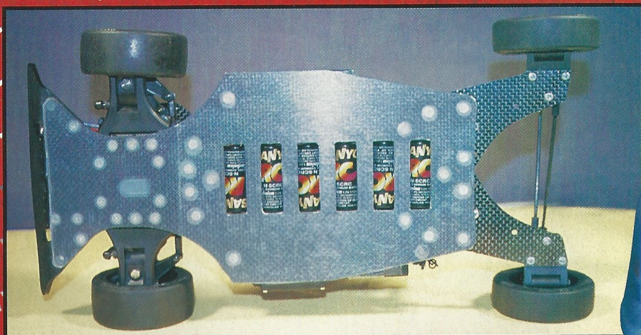
You can see the in-line layout of the nicads, note the Associated covering for the bottom of the chassis, saves all that kerbing damage.
