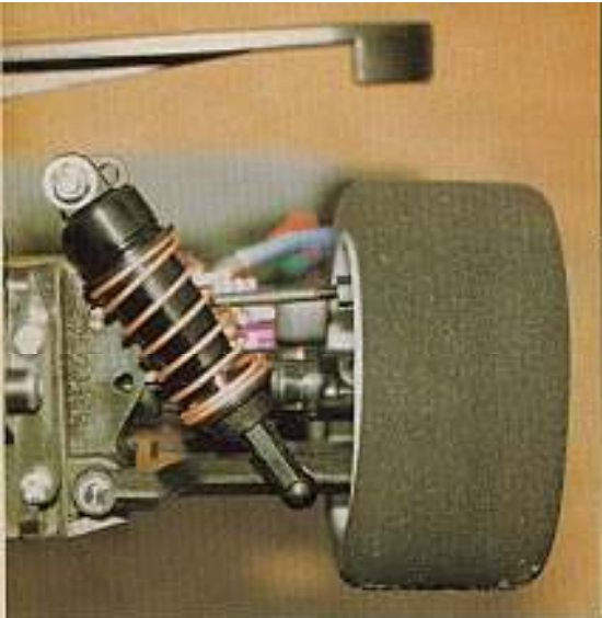
⓪ Rear oil-filled shock absorbers.
