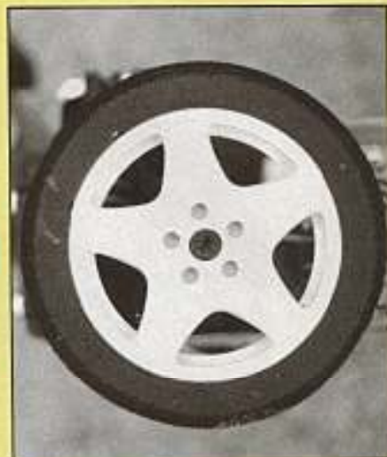
○ Nicely moulded wheels with foam/rubber tyres.
