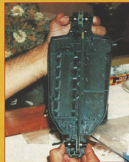
The chassis tub with the front, rear diffs and drive belts fitted
