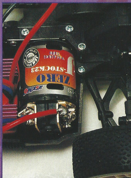
Yokomo Zero J Stock motor crowding out the Novak Explorer II Speedo
