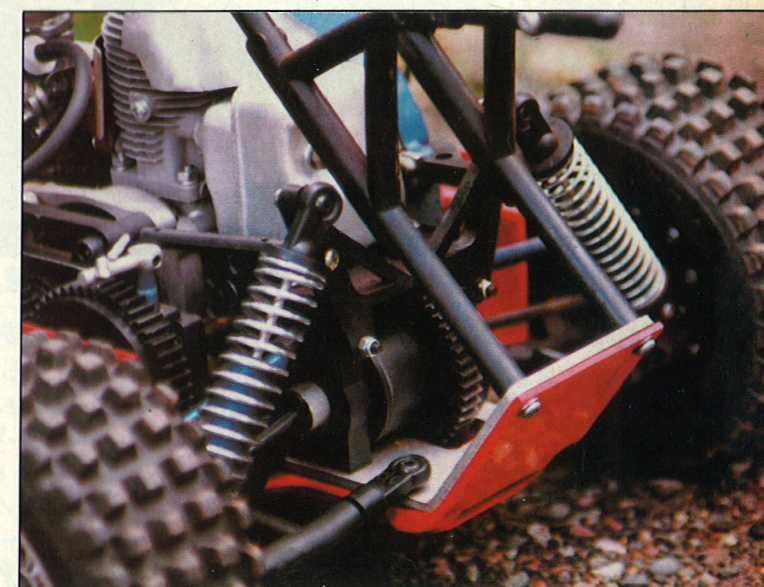
Left, Kawasaki's 23cc engine was specially developed for this car and can be tuned for as little as £45.00 to give just under 4 bhp.
