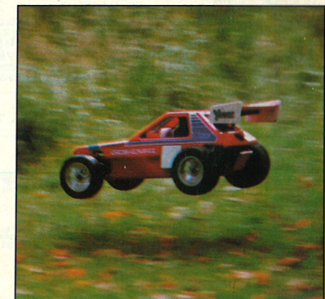
Left, Kawasaki's 23cc engine was specially developed for this car and can be tuned for as little as £45.00 to give just under 4 bhp.
