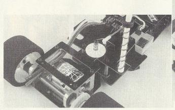
Magic Johnson gears and ball diff completes the rear end. A sliding damper system is fitted for tuning the handling. Firm body posts are included with adjustable height positions. In the UK the kit will comes with a BMW 3 series body and will be available as a rolling chassis or complete with Spec motor and battery.
