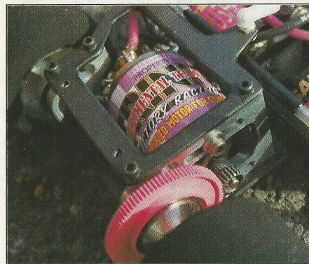
The rear pod is so designed to allow the maximum access to the motor and wires.
