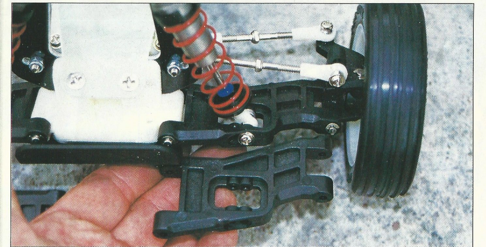
Right: The shorter arms in comparison with the standard front end.
