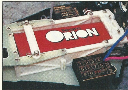
The battery crate is really only suitable for stick pack cells.
