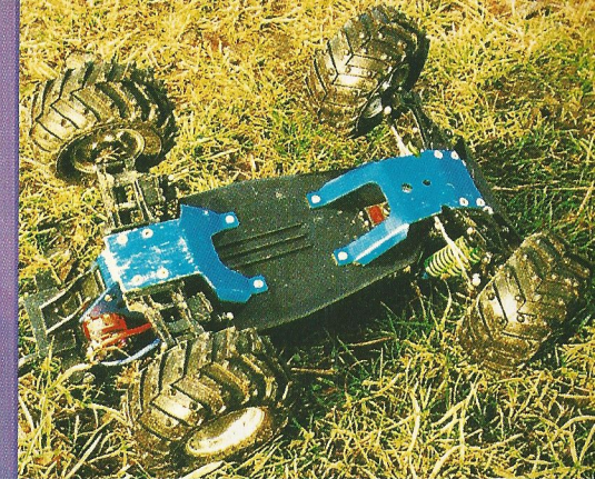
The well used under shields
