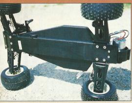
The moulded 'U' shaped chassis means the heavy battery pack sits low down, whilst the raised sides give good ground clearance.
