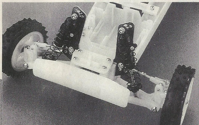
Right; Telescopic drive shafts are neat, light and require hardly any maintenance. Right; Plenty of suspension movement from the long rear wishbones.
