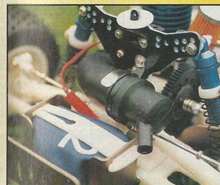
The stubby exhaust pipe and rear battery box.
