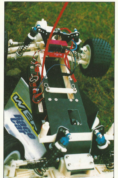
A general view along the chassis. The cells drop through the upper plate and are retained by the nylon cross bar and a lip under the speed controller. The moulded 'gates' that make up the box chassis design can be seen through the cell aperture.
