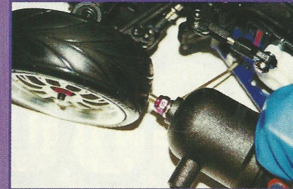
One small snag that needed to be sorted, the screw on the front of the exhaust fouls the front wheel on full lock
