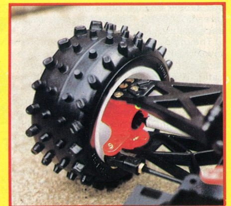
Knobby tyres are supplied for all four wheels. The steering arm can also be seen, this is identical at front and rear.
