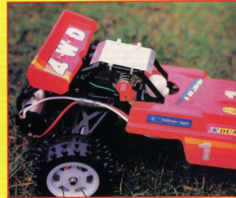
A sturdy roll-cage neatly covers the resistor, speed controller and driver figure, the rest of the car is covered with a moulded red lexan body and aerofoil.
