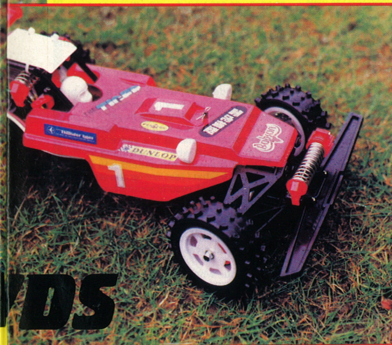
Coil over oil filled mono shock absorbers are used at both ends, giving adequate suspension movement.
