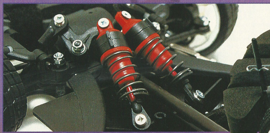
The pushrod operated inboard front suspension remains, diff cover hides new ball diff
