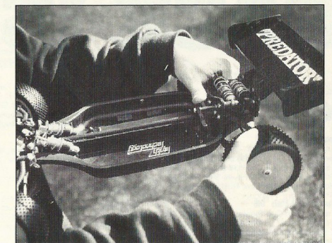
Checking the adjustment of the rear diff.
