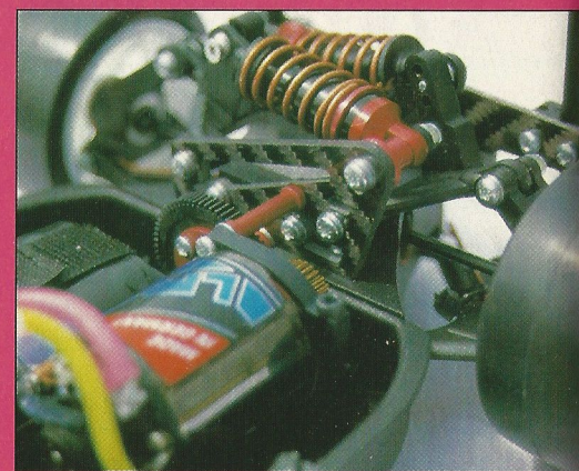
The racing team spec teardown now comes with the pure carbon suspension plates. All the alloy parts are now anodised red.
