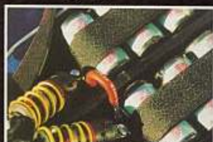
The link wire for the coil packs has to be kept clear of the carbon prop shaft
