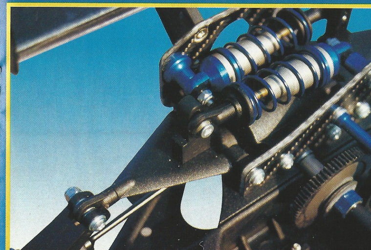
The inboard rear suspension set-up. By raising or lowering the shock's outer pick-up point on the wishbone's 'tower,' the damping/springing can be altered. Neat and accessible.
