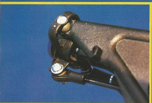
The kingpin's lower balljoint housing is now an integral part of the lower wishbones. The camber angle is now adjusted at the top only.
