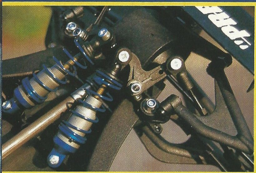
The front end is as adjustable as the rear, three alternative positions on the rocker cranks allowing the driver to dial in understeer or oversteer at will.
