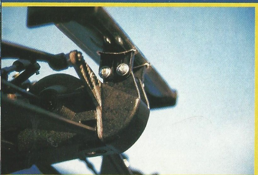
'Digging-in' when landing off a jump is now a thing of the past, thanks to the new, shorter, rounded off nose cone.
