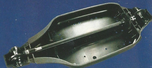
The moulded chassis isn't the only new feature on the International - the integral transmission casings house redesigned differentials using much beefier, moulded gears with larger, stronger teeth.
