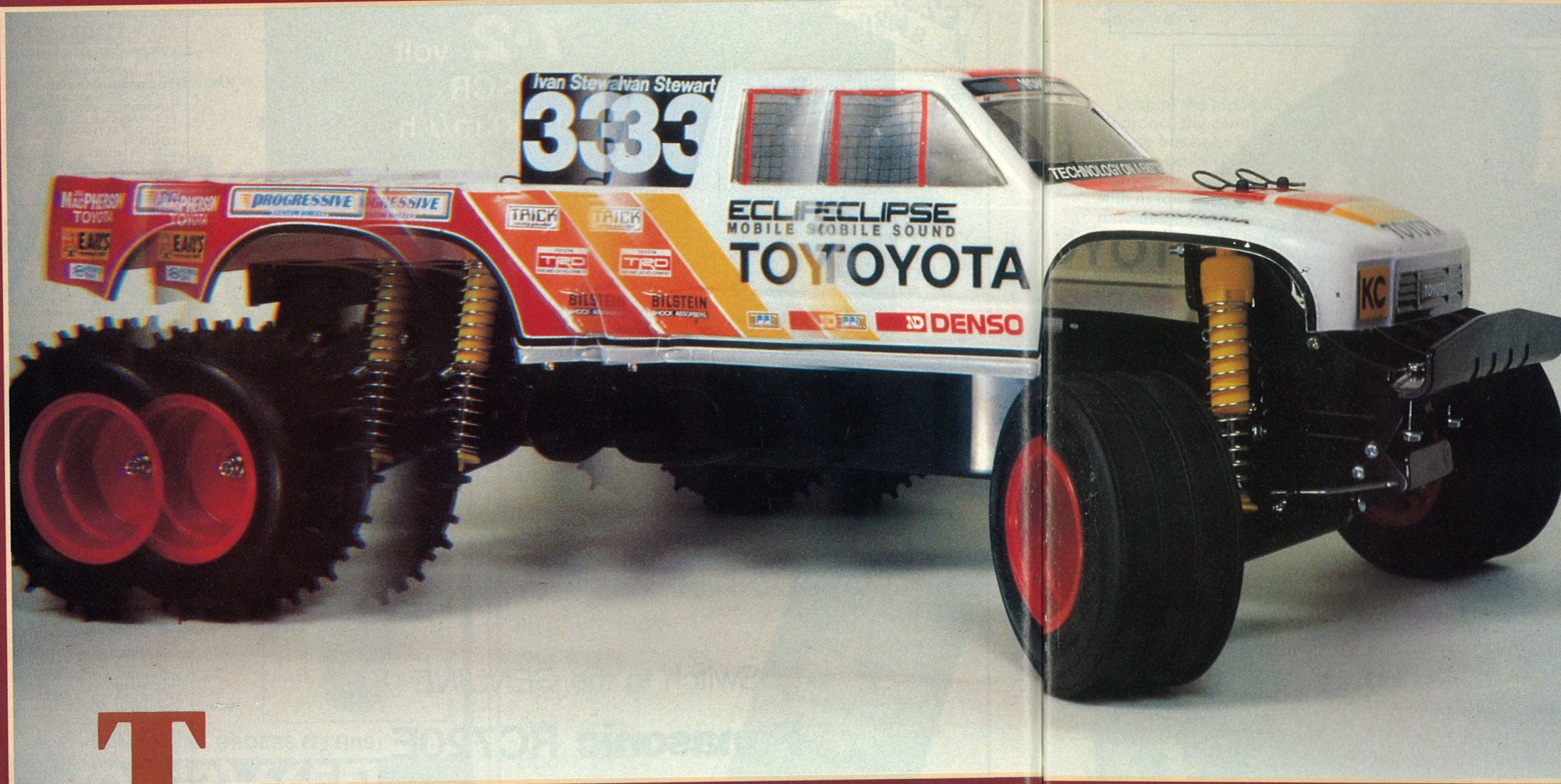
The Toyota Truck consists of a King Cab chassis & the new racing style Hi-Lux bodyshell.
