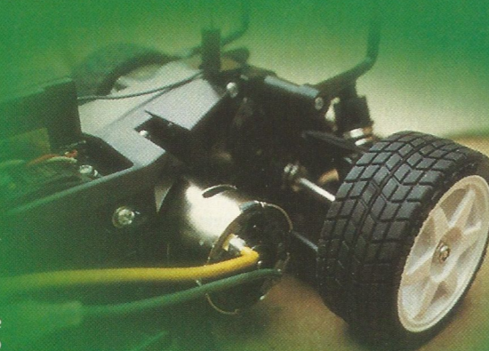
The neat and tidy front suspension detail
