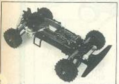
Below, clockwise: The front suspension has plenty of "movement" and has the facilities to fit two separate shock absorbers. The speed controller supplied in the ThunderShot is that of the standard 3-step type. The suspension arms are moulded from tough blue plastic. The radio crate is formed from light plastic to give a purposeful chassis box section. The radio equipment is protected by a lean oversay. The new one-piece flat face plastic wheels certainly look purposeful. The new futuristic shell tops the car off well to give a purposeful look. The rear end is sprung by two of Tamiya's CVA shocks. Finally the new front bumper is neat and strong.
