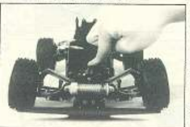
Below, clockwise: The front suspension has plenty of "movement" and has the facilities to fit two separate shock absorbers. The speed controller supplied in the ThunderShot is that of the standard 3-step type. The suspension arms are moulded from tough blue plastic. The radio crate is formed from light plastic to give a purposeful chassis box section. The radio equipment is protected by a lean oversay. The new one-piece flat face plastic wheels certainly look purposeful. The new futuristic shell tops the car off well to give a purposeful look. The rear end is sprung by two of Tamiya's CVA shocks. Finally the new front bumper is neat and strong.
