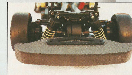
A very nice urethane sponge front bumper is provided and suits most Tamiya shells
