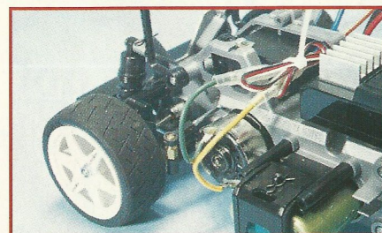
As with the diff, the motor and battery become part of the chassis members thanks to clever design.
