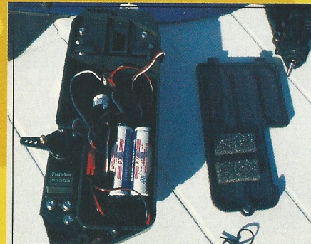
Radio box detaches with the servos for cleaning
