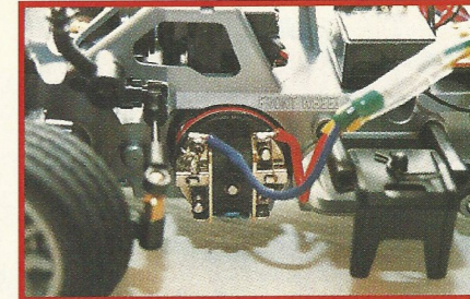
Motor is located just ahead of the battery.
