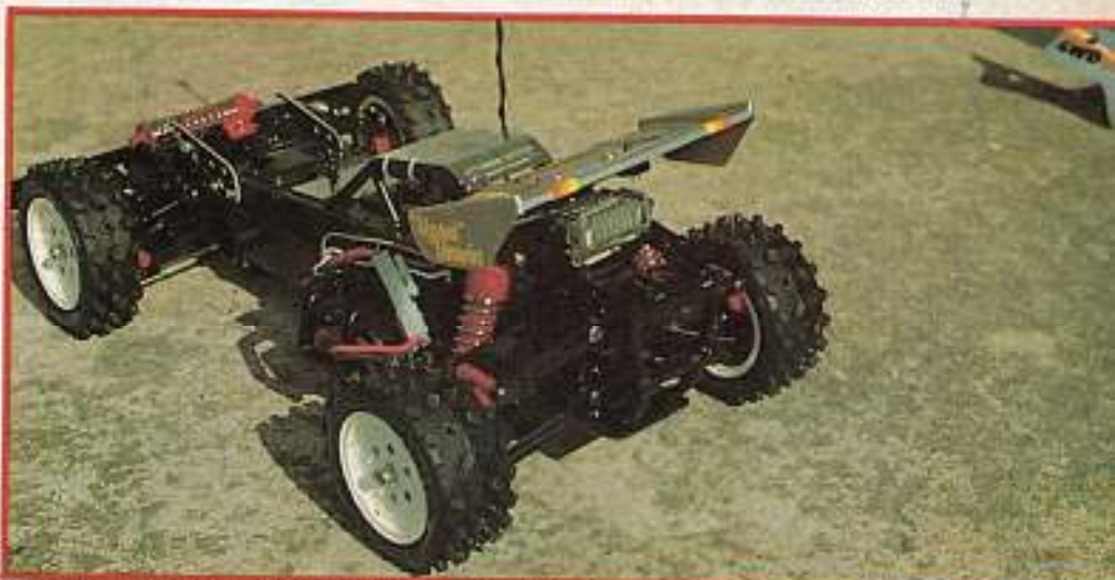
Rear view shows the double wishbone rear suspension.
