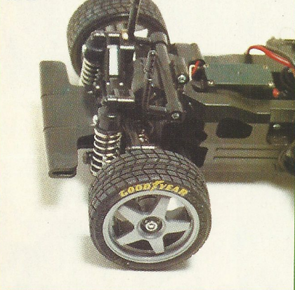
You can see this is the front, it has a steering servo
