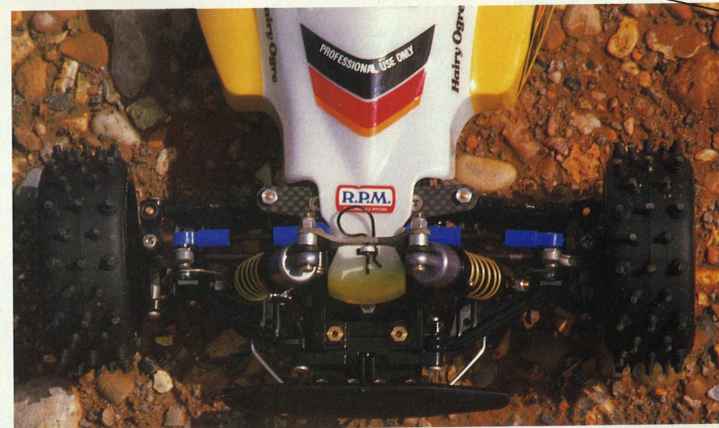
Lightweight very smooth shocks and complicated anti-roll bar, adjustable wing mount.
