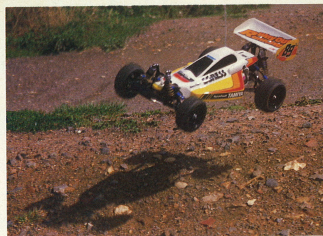
Lightweight very smooth shocks and complicated anti-roll bar, adjustable wing mount.
