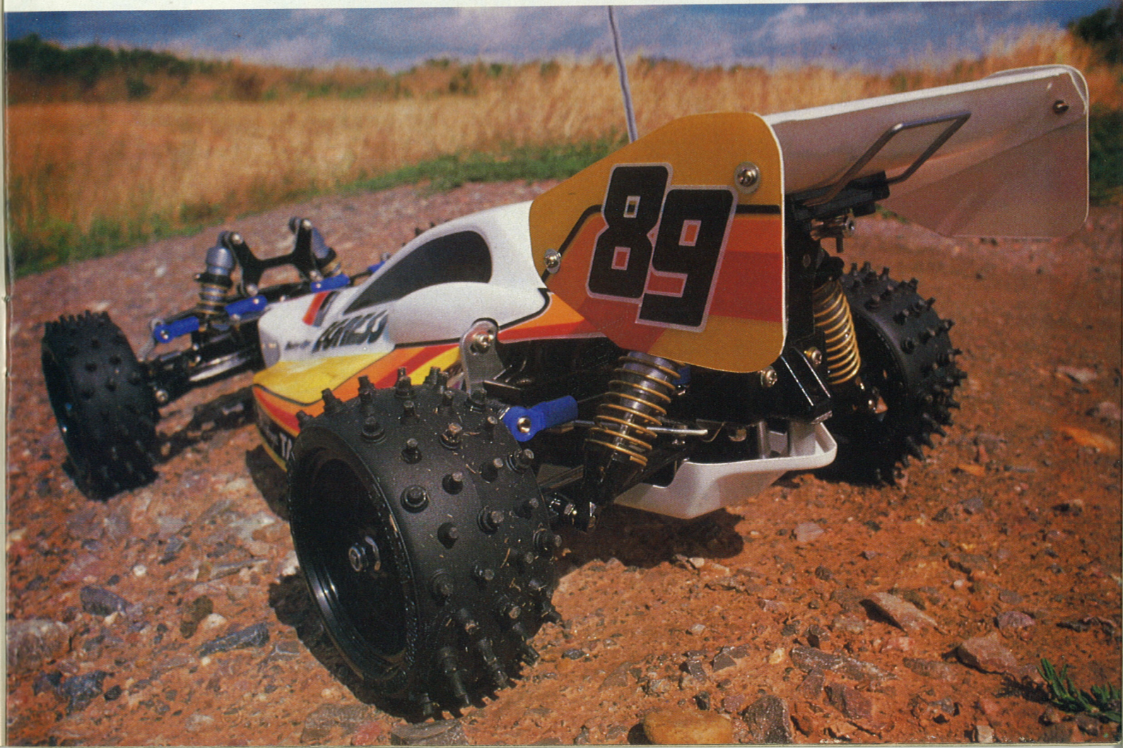
Top: black wheels, a la Vanquish, all-encompassing undertray which matches smart body, held in situ with split pins and Velcro.
