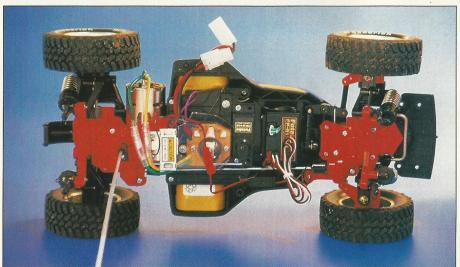
Once a budget priced 2ch radio set has been purchased, the Chevy's kit provides every other item needed to get it rolling apart from the battery pack. The mechanical wiper board speed controller is clearly seen here above the 7.2v battery pack.
