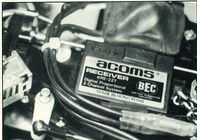
BEC receiver and resistors for speed controller protected by rubber cover.
