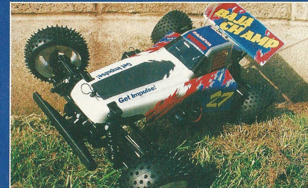
The only modification allowed for Cadet racing - ball races replace the white plastic bushes - a worthwhile investment
