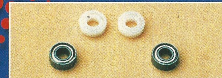
The only modification allowed for Cadet racing - ball races replace the white plastic bushes - a worthwhile investment
