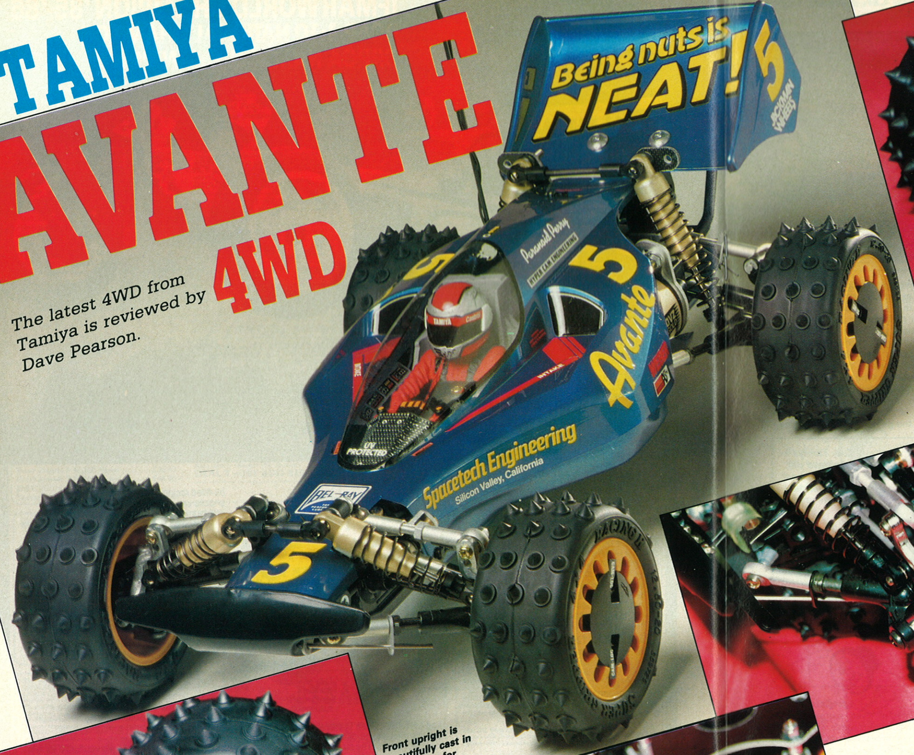
Left and above, suspension borrows heavily from formula one cars of not so long ago, note those beautiful rose joints.
