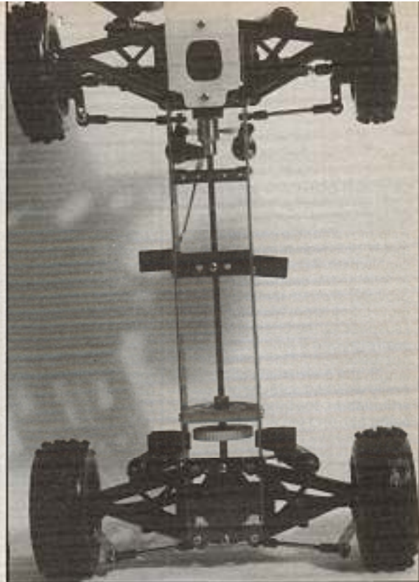
Left: The front hubs are moulded in plastic - note adjustable suspension link for camber alteration. Above: Plenty of room for radio equipment.
