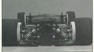
Left; The car is supplied with saddle pack trays. Top; Front suspension is fully adjustable for camber and castor. Bottom Left; Tenforce uses belt drive and will require the purchase a set of pinions.
