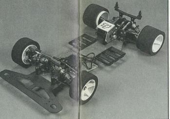
Tenforce does suffer from a small amount of bump steer, although this seems not to affect the handling. Centre; All track rads are supplied, and the fits are excellent. Note the well designed body mounts (firstly seen on a Japanese Kit).
