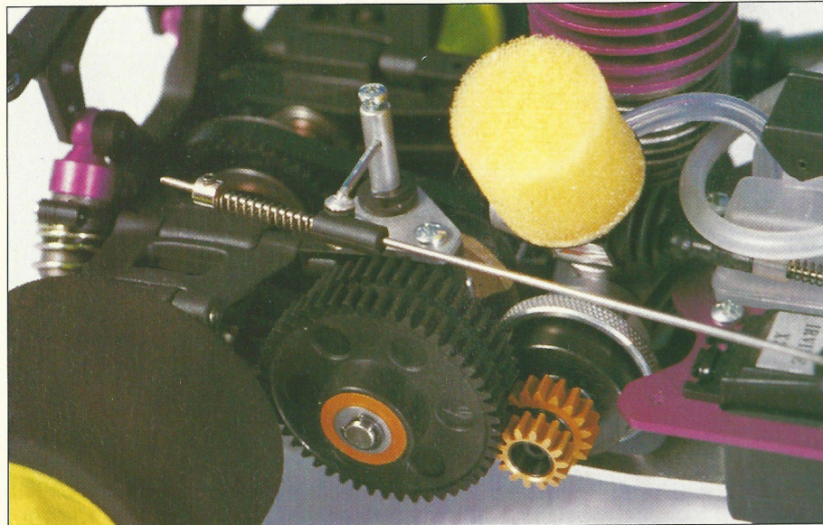
The effectiveness of the brake is easily adjusted by the strength of the spring, or the amount of compression set by the collet.
