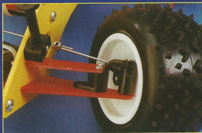
Under the Mini body shell is found a simple two piece plastic chassis and new stronger drive system. 540 motor sits at the rear and with encouragement the car will pull a full blown wheelie!
