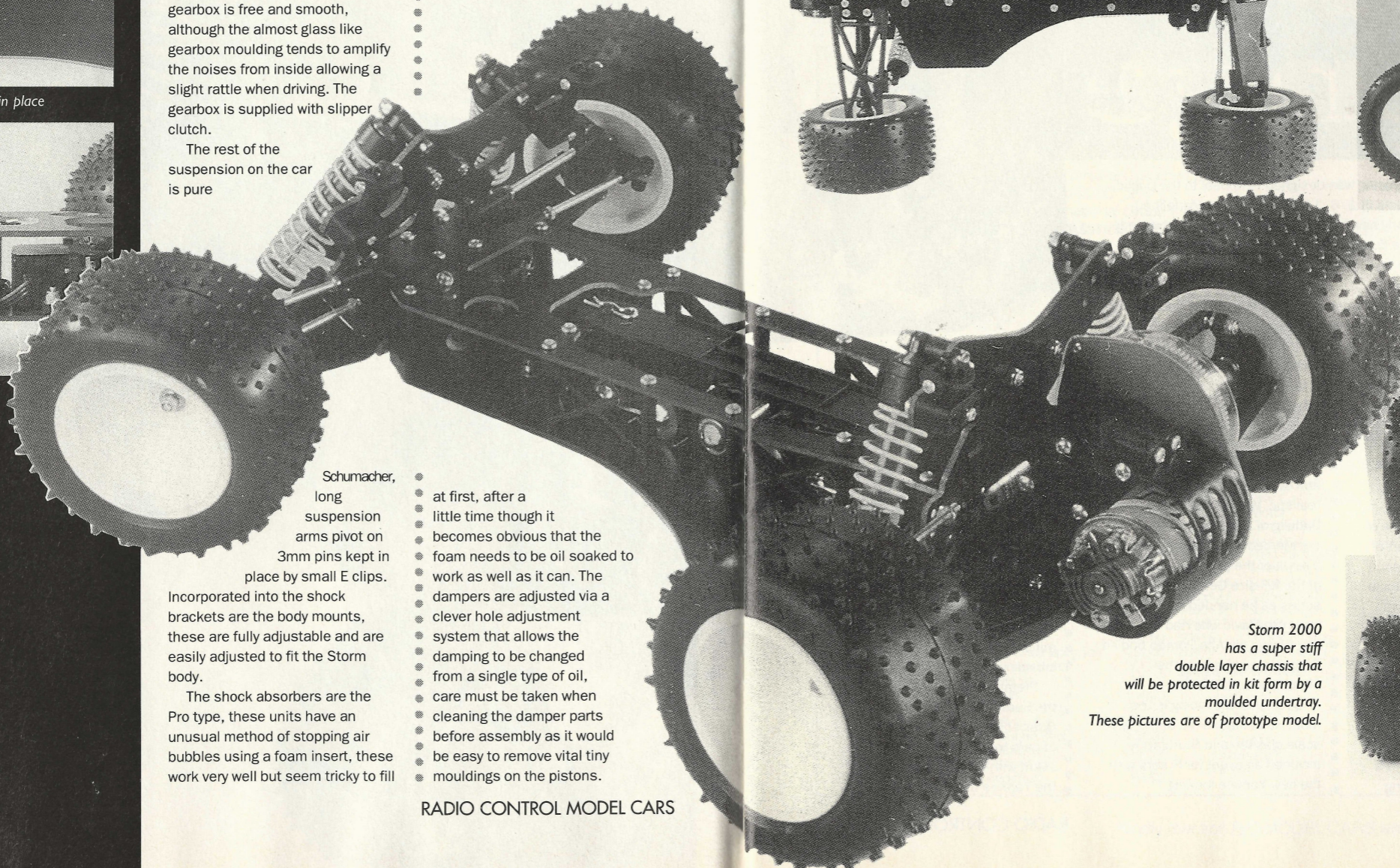
New wheels have very low flex, are light and smooth to resist mud and dirt!
