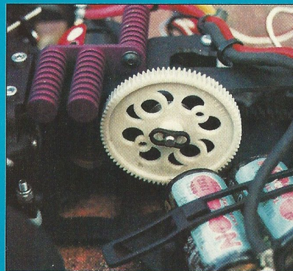
Left: A neat cup holds the spur gear, quick changes are now on.
